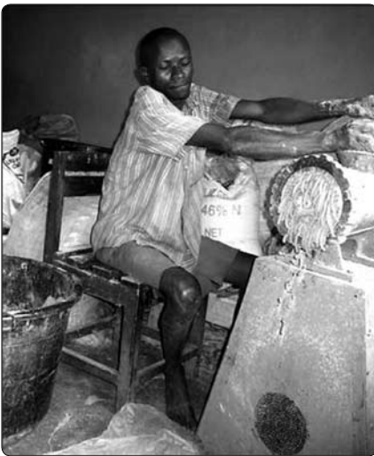
Figure 4.3-3. A simple pelleting machine is used to prepare fish feeds on the farm at Sagana Aquaculture Centre.
