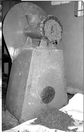
Figure 4.7-2. A home-made feed from a pellet machine.
