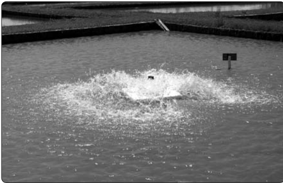
Figure 4.7-5. An electrical aerator.
